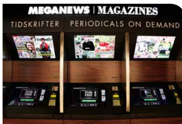
The MegaNews kiosk houses a colour touchscreen display, card reader, Ricoh ProC 751 colour printer and EFI Fiery server.
